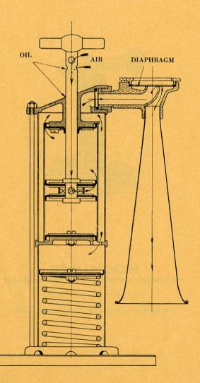
**PUMP.** The leather packings of the pump should be kept well oiled. This is done when necessary by injecting the thinnest lubricating oil (e. g. sewing-machine oil) through intake openings in the pump rod as well as on the edge between the pump rod and the pump. The oil is then distributed by pumping vigorously and turning the pump rod.
