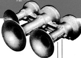
**M3** A smaller unit than the M5, but a fully efficient warning signal which produces a balanced tone of the three combined bells, of sufficient range and volume for general freight or switcher service. Somewhat less euphonious in sound than the M5, but more than adequate for its purposes. No more than the original three bells may be mounted on this base. Weighs 28 pounds. Uses bells 1, 2, and 4.
